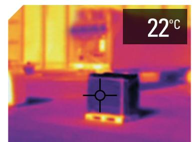
Test conditions: covered pallets on simulated tarmac in Lakeland, FL, November 2012 at ~11 a.m. Full sun with ambient temperature at 20°C.
